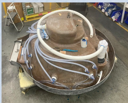
FIGURE D: Spillover right side/ride side if viewing from the back of standard spa: Water filtration connected near the steps; connected to the suction/return lines.
