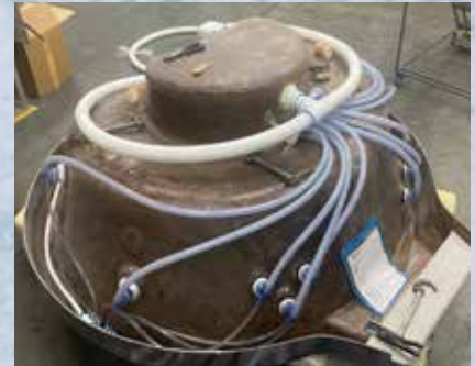
FIGURE C: White suction and return lines run from canister (top) to connect to the pool.
