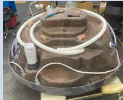
FIGURE E: Step view- Suction and Return lines for pump hookup/ Cardinal pool connection
