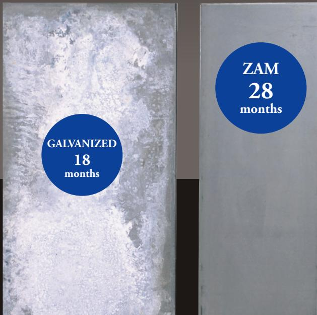
Cardinal is proud to offer ZAM®—the most effective non-corrosive coating for steel panels & steps in the industry. ZAM® is a hot-dip coated steel sheet that has a layer of **Zinc, 6% Aluminum, and 2% Magnesium**. The effects of magnesium and aluminum together allow our ZAM® coated steps to have excellent corrosion resistance, scratch resistance, and formability.
